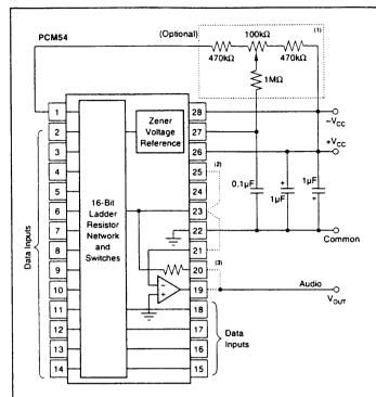
NOTES: (1) MSB error (BPZ differential linearity error) can be adjusted to zero using this external circuit. (2) Connect to bipolar operation (+V  $_{CC} \geq$  8.5V for unipolar operation). (3) Connect for V  $_{OUT}$  operation. When V  $_{OUT}$  amp is not being used (I  $_{OUT}$  mode), terminate with an external  $3k\Omega$  feedback resistor between pin 19 and pin 21, and a  $1k\Omega$  resistor between pin 21 and pin 22 to reduce possible noise effects.
