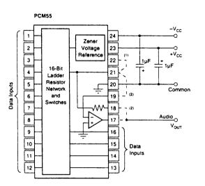
NOTES: (1) Connect for bipolar operation. (+V  $_{CC} \ge 8.5 V$  for unipolar operation). (2) Connect for V  $_{OUT}$  operation. When V  $_{OUT}$  amp is not being used (I  $_{OUT}$  mode), terminate with an external  $3k\Omega$  feedback resistor between pin 17 and pin 19, and a  $1k\Omega$  resistor between pin 19 and pin 20 to reduce possible noise effects.
