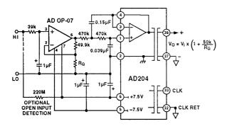
Figure 17. Input Amplifier & Filter for Sensor Signals
