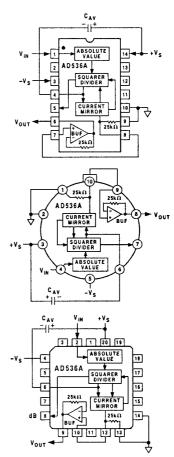
Figure 1. Standard RMS Connection
