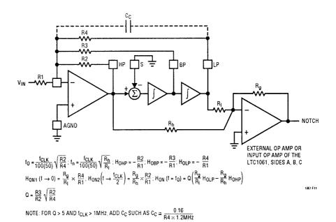
Figure 11. Mode 3a: 2nd Order Filter Providing Highpass, Bandpass, Lowpass, Notch
