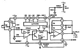
Figure 2. 0 V to +10 V Unipolar Voltage Output
