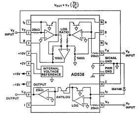
Figure 12. One-Quadrant Combination Multiplier/Divider By simply connecting the input  $V_X$  (Pin 15) to the +10 V reference (Pin 4), and tying the log-ratio output at B to the antilog input at C, the AD538 can be configured as a one-quadrant analog multiplier with 10-volt scaling. If 2-volt scaling is desired,
