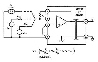
Figure 7. Connections for Summing or Current Inputs
