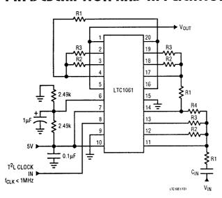
Figure 1. the 6th Order LP Butterworth Filter of Figure 5 Operating with a Single 5V Supply.
