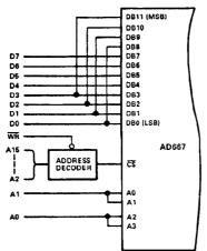
Figure 9. Right-Justified 8-Bit Bus Interface
