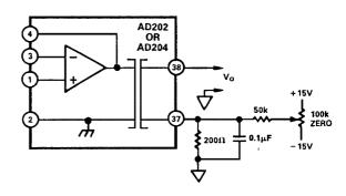
Figure 9. Output-Side Zero Adjustment
