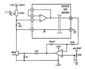
Figure 19. High-Compliance Current Source
