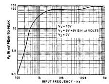
Figure 7. Vy Feedthrough vs. Frequency
