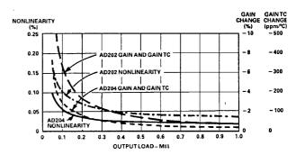
Figure 2. Effects of Output Loading
