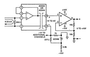
Figure 18. Process Current Input Isolator with Offset
