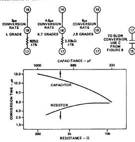
Figure 6. AD578 Conversion Times vs. R or C Values
