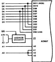
Figure 8. Left-Justified 8-Bit Bus Interface
