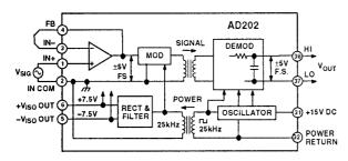
Figure 1a. AD202 Functional Block Diagram
