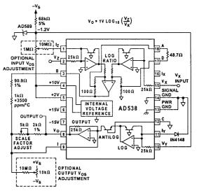
Figure 14. Log Ratio Circuit
