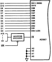
Figure 10. Connections for 12- and 16-Bit Bus Interface
