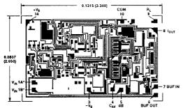
PAD NUMBERS CORRESPOND TO PIN NUMBERS FOR THE TO-166 14-LEAD CERAMIC DIP PACKAGI
