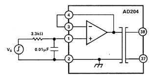
Figure 12. Input Filter for Improved Step Response
