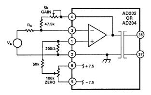
Figure 8b. Adjustments for Summing or Current Input
