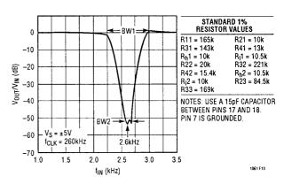
Figure 13. Resistor Values and Amplitude Response of Figure 12 Topology. The Notch is Centered at 2600Hz.
