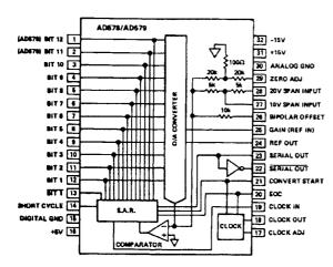
Figure 1. AD578/AD579 Functional Block Diagram and Pinout
