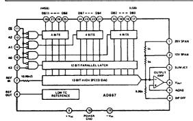
Figure 5. AD667 Block Diagram
