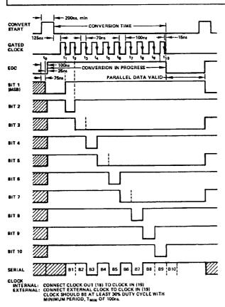
Figure 2b. AD579 Timing Diagram
