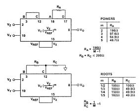
Figure 15. Basic Configurations and Transfer Functions for the AD538
