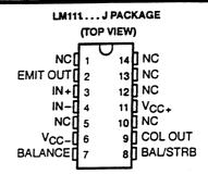
LM111 ... JG PACKAGE LM211, LM311 ... D, DB, P, OR PW PACKAGE (TOP VIEW)
