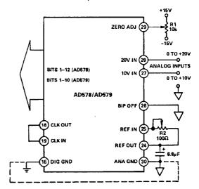
Figure 3. Unipolar Input Connections
