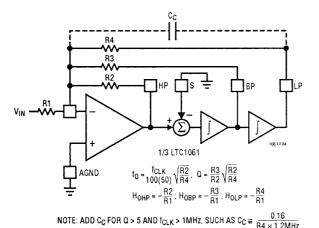
Figure 4. Mode 3: 2nd Order Filter Providing Highpass, Bandpass, Lowpass
