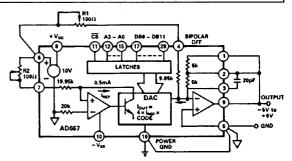
Figure 3. ±5 V Bipolar Voltage Output
