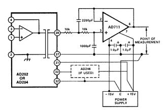
Figure 13. Output Filter Circuit Showing Proper Grounding
