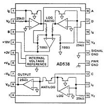
Figure 9. Functional Block Diagram
