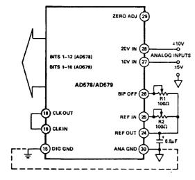
Figure 4. Bipolar Input Connections
