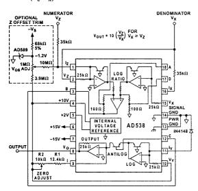
Figure 13. Two-Quadrant Division with 10 V Scaling
