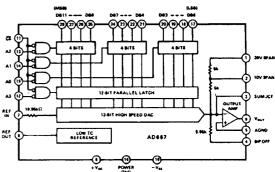
The AD667 is available in five performance grades. The AD667 J and K are specified for use over the 0 LC to +70 LC temperature range and are available in a 28-pin molded plastic DIP (N) or PLCC (P) package. The AD667S grade is specified for the -55 LC to +125 LC range and is available in the ceramic DIP (D) or LCC (E) package. The AD667A and B are specified for use over the -25 LC to +85 LC temperature range and are available in a 28-pin hermetically sealed ceramic DIP (D) package.
