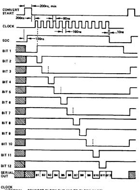
CLOCK INTERNAL: EXTERNAL: CONNECT CLOCK OUT (18) TO CLOCK IN (19) CONNECT EXTERNAL CLOCK TO CLOCK IN (19) CLOCK HOOLUD BE AT LEAST 30% DUTY CYCLE WITH MINIMUM PERIOD, T<sub>MIN</sub> OF 100ns.
