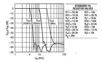
NOTE: ADD A CAPACITOR C ACROSS  $R_g$  TO CREATE A 7TH ORDER LOWPASS SUCH AS  $(1/2\pi R_g C)$  = (CUTOFF FREQUENCY)  $\times$  0.38
